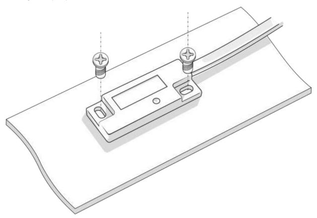
The element to which the sensor is attached should be rigidly connected to the body of the vehicle. Fastening to flexible, soft or deformable elements (e.g. to wire harnesses) will cause false alarms from the tilt sensor and will prevent the shock sensor from working.
